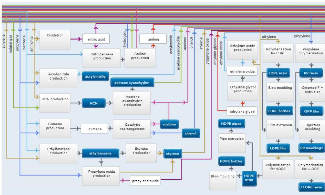
**Figure n.3:** flow diagram - Process data set: Polyethylene film (PE-LD); technology mix; production mix, at producer – Source: GaBi 6
